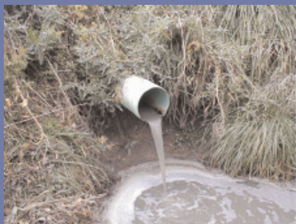
Figure 3. Contamination of subsurface drainage effluent attributable to heavy rainfall following application of liquid swine manure to an untilled, corn silage field in Darke County, Ohio. Analysis of the effluent indicated a BOD 5 of 3200 mg/L, 205 mg NH 4 -N/L, 9.0 mg NO 3 -N + NO 2 -N/L, and 174 mg total P/L. Courtesy of OEPA.
