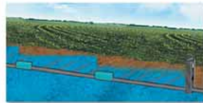
Side view of how Inline Water Level Control Structure and Water Gates "Stair-Step" water up through the soil profile.
